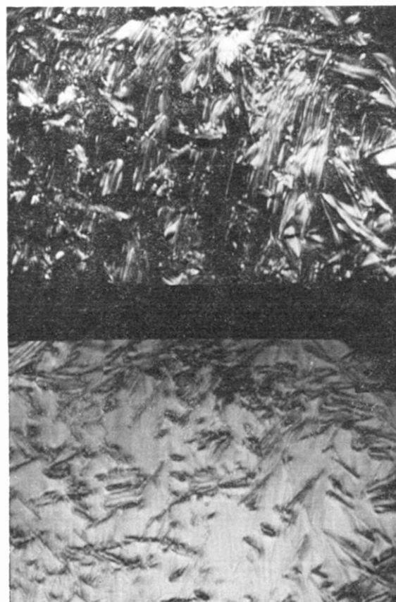
Figure 6 Photomicrograph of the growth of extended-chain crystal at the same condition a few minutes after that of Figure 5. The striations change colour with time and perfect extended-chain crystals are formed rapidly
