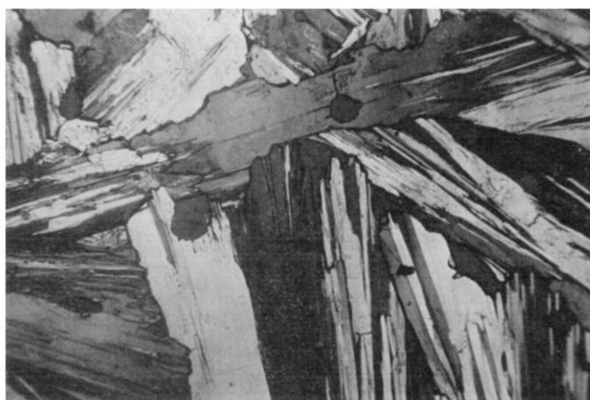
Figure 7 Photomicrograph of pure 1,2,4,5-tetrachlorobenzene crystals; magnification 20 diameters
