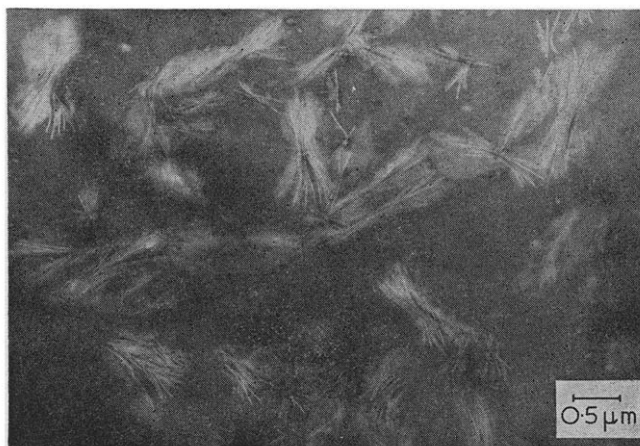
Figure 5 Spherulitic morphology obtained by crystallizing at 1 kbar and 0°C, for 2 h. Note the growth of the lamellae in the 'side-on' position
