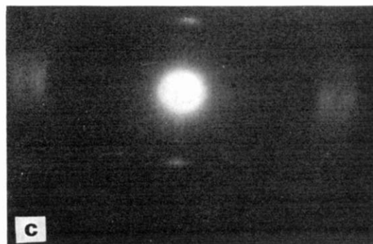
Figure 2 X-ray photographs of (a) 'normal nylon-6' and (b) and (c) 'special nylon-6' slow rolled at room temperature and fast rolled at: (b) 150°; (c) 195°C
