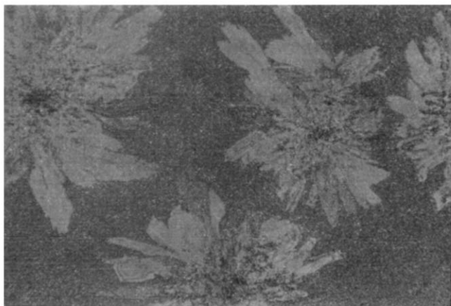
Figure 10 Photomicrograph of the spherulitic structures developed during simultaneous growth of polyethylene and 1,2,4,5-tetrachlorobenzene, at 105°C; magnification 46 diameters
